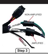
If the vehicle is equipped with a factory amplifier, connect the 8-pin connector to the AMPLIFIED connector. All others connect to the NON AMPLIFIED 8-pin connector.
