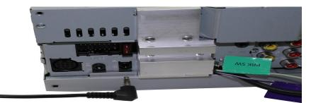
4. Connect the 14 way molex connector to the interface
