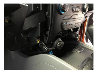
Step 4 The storage panel can be removed by pulling the trim towards you. This will reveal the final 2x 7mm bolts scuring the radio's front panel to the dash.
