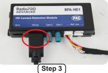
Connect one end of the 12" HDMI cable into the HD OUT port on the HD1 interface module. The other end will be connected to the HDMI input port on the Stinger radio module after mounting the HD1 interface module into the vehicle.
