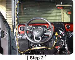
Route the GPS cable down the A-pillar past the plastic dash side panel, then route the cable behind the lower dash below the steering column and then up the center stack to the radio opening. (Secure with zip ties along the way.)
