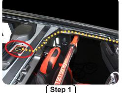
Clean the area next to the factory antenna on the center roll cage structure and stick the GPS mounting plate to it. Then, secure the GPS antenna to the mounting plate (it is magnetic). Route the cable behind the trim panels of the roll cage over to the driver side A-pillar.
