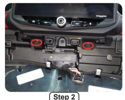
Connect the Stinger display cables into the back of the Stinger radio display and secure it to the radio unit mounting bracket against the dash using the orange clips and the two 7mm screws below the radio cavity.
