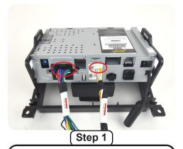
Connect the two Stinger radio module connectors which are labeled "16PIN RADIO" and "10PIN RADIO" into the appropriate ports on the Stinger radio module.
