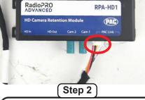
Connect one end of the 18" harness (10P-2-10P-18) into either of the two 10-pin PAC Link ports on the RPA-HD1 interface module. The other end will be connected to the open 10-pin port on the PL1 interface module after mounting the radio unit into the vehicle.
