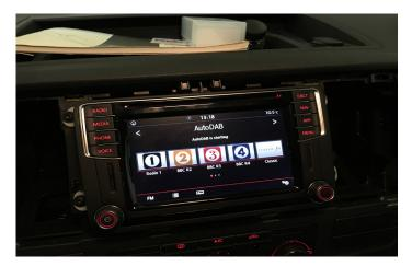
3. Pull the radio towards you in order to free it from the dashboard, unplugging the connectors on the rear of the radio.
