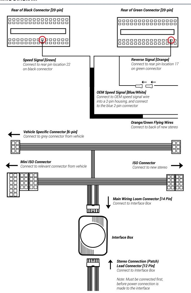
The following diagram, though based on careful research, is an example only. Individual steering wheel control configurations may differ.
