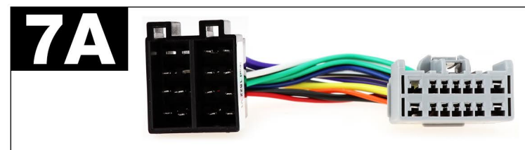
7A When dealing with an ISO vehicle connector, opt for LEAD 1822 as shown. Connect the grey plug to the Land Rover connector in image 7 and the ISO connectors to the corresponding female ISO port above.
