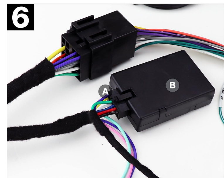
6 ISO connector and CAN interface. Plug the 12 pin molex (A) in to the CAN interface (B) and plug the ISO (male) connector from the CAN104-LR01 harness in to the UN1810E Power lead (ISO female)
